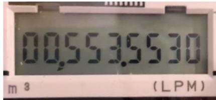
**Rate:** When the screen toggles to a different display, the rate of flow is shown. This will display for four seconds. The display will then toggle back to the read screen. Each additional read screen will display for eight seconds.
