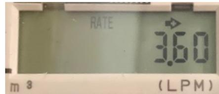
The number displayed on the “reading” screen is used for billing purposes and is the number we require. Include the decimal point if there is one. Please do not provide the “rate” number.
