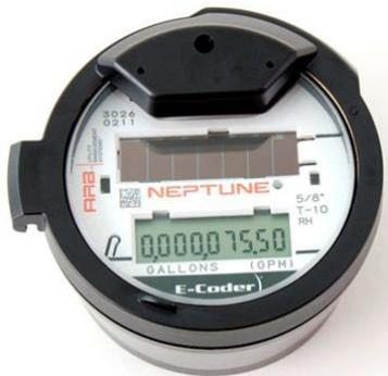
To read your meter, shine a bright light such as a flashlight on the screen and the display will activate. When activated, the display will first show a segment test.
