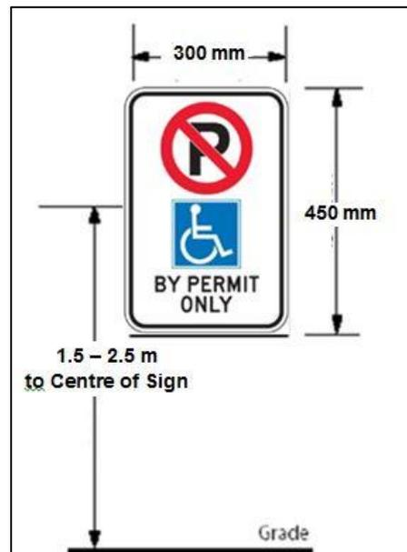
Figure 6 - Sign Installation
